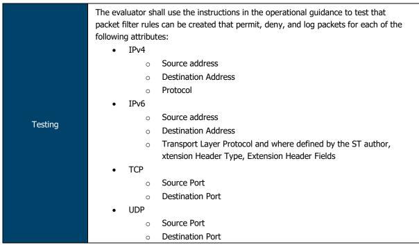
The evaluators constructed and tested numerous packet filtering rules that exercised each of the protocols, attributes and reactions listed in this requirement. The evaluators confirmed that, for each configured rule, the TOE behaved as expected and audit logs were generated appropriately.
